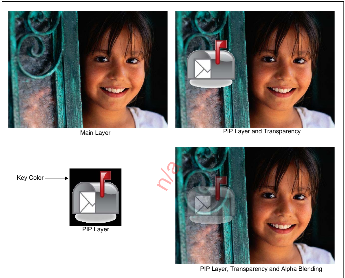
Figure 14-3: PIP Layer Alpha Blending
